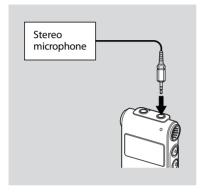
1 Connect an external microphone to the **\*** (microphone) jack when the IC recorder is in the stop mode.
